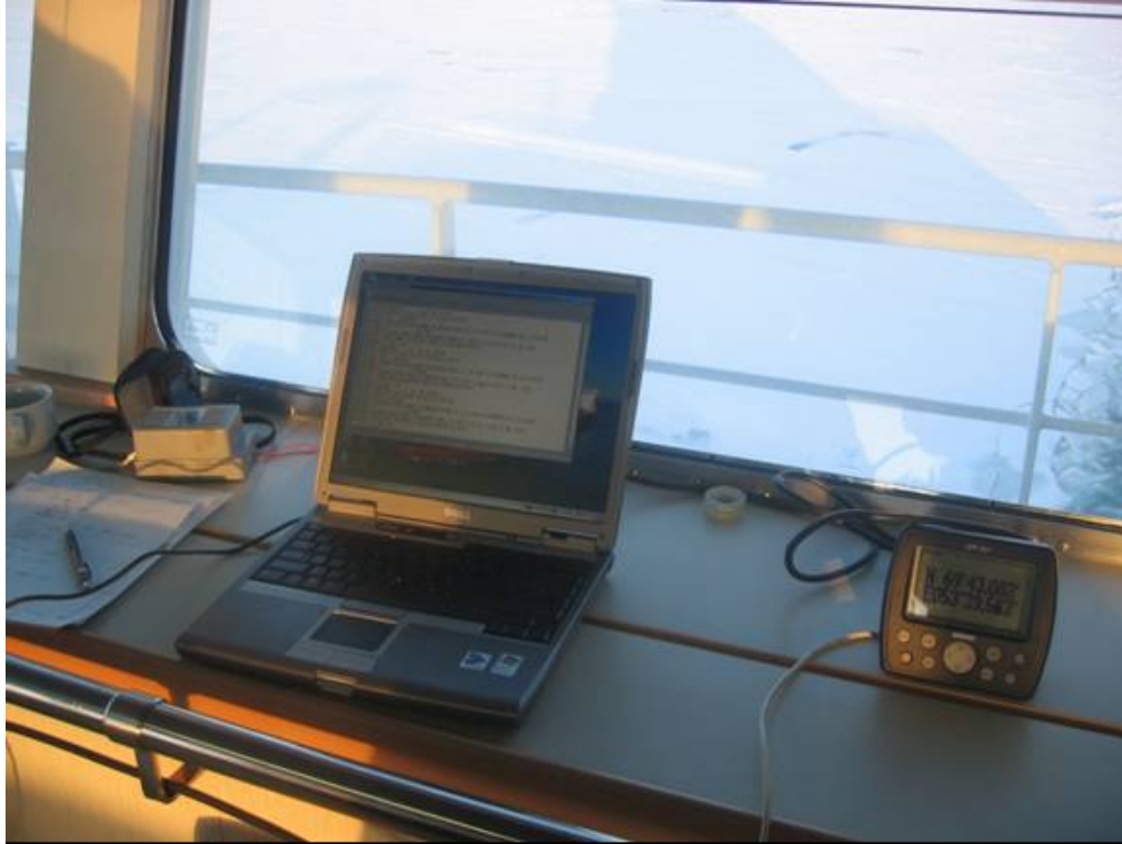
Figure 4-1 GPS receiver and workstation on the bridge
