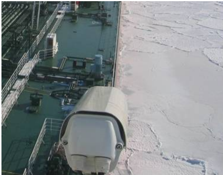
Figure 4-2 AARI digital video camera recording vertically turning ice cusps
