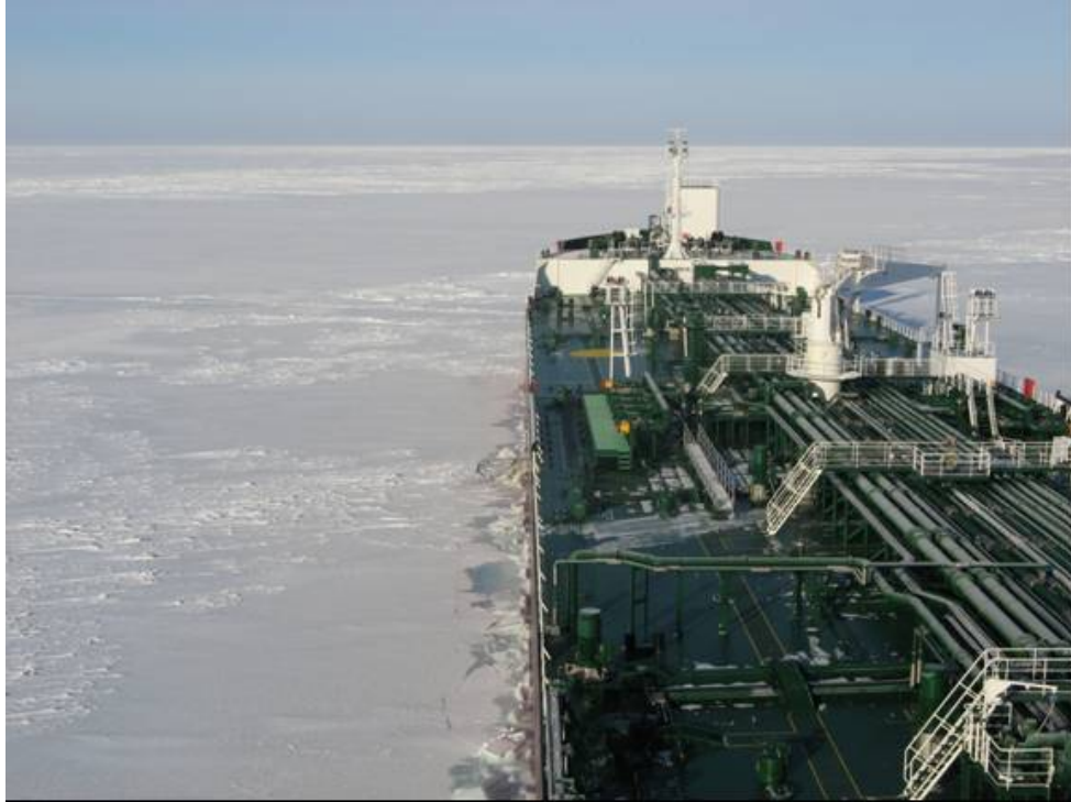
Figure 2-2. Typical ice conditions of the performance tests (March 20, 2008. Speed-power test, 30 cm)
