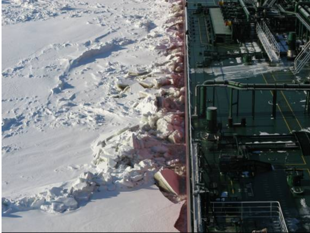
Figure 2-4. Bollard pull test in a cluster of ridges
